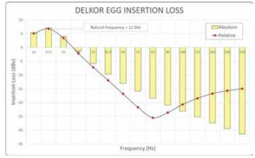
Relative Insertion Loss Reference Track – 150kN/mm
